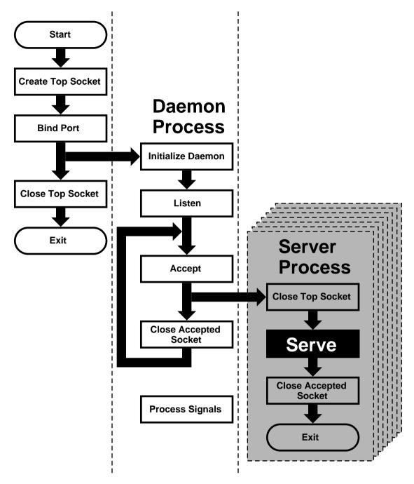
We moved the *serve* from the *daemon process* to its own *server process*. However, because each child process inherits all open files (and a socket is treated just like a file), the new process inherits not only the "*accepted handle*," i.e., the socket returned by the accept call, but also the *top socket*, i.e., the one opened by the top process right at the beginning.
